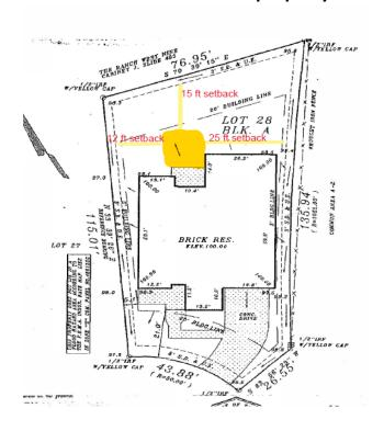
Scaled site plan example with setback measurements from all sides of project to all property lines. The scaled site plan should be with your closing documents from when you purchased the home.
